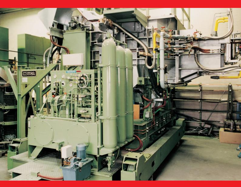
The production of vertically casted non-ferrous special alloys demands not only a highly developed continuous casting technique but also an alloying and casting furnace which is capable of supplying a homogeneous melt over the whole casting time under defined conditions with exact alloy quality and temperature control.
