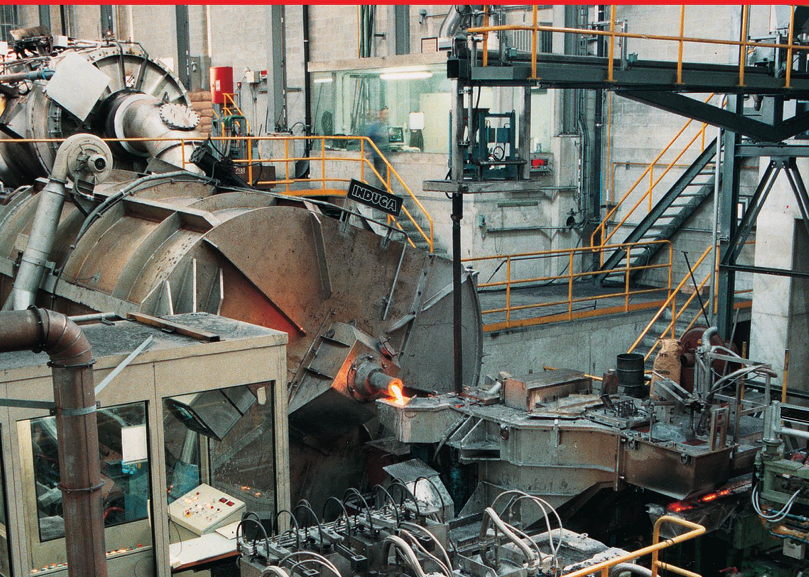
This induction heated alloying and metering furnace is a useful alternative solution to a conventional unheated tundish system. A very precise alloy adjustment, for example during the production of low-phosphorous DHP copper, combined with a good mixing and complete homogenisation of the melt are fundamental for casting high-quality copper grades
