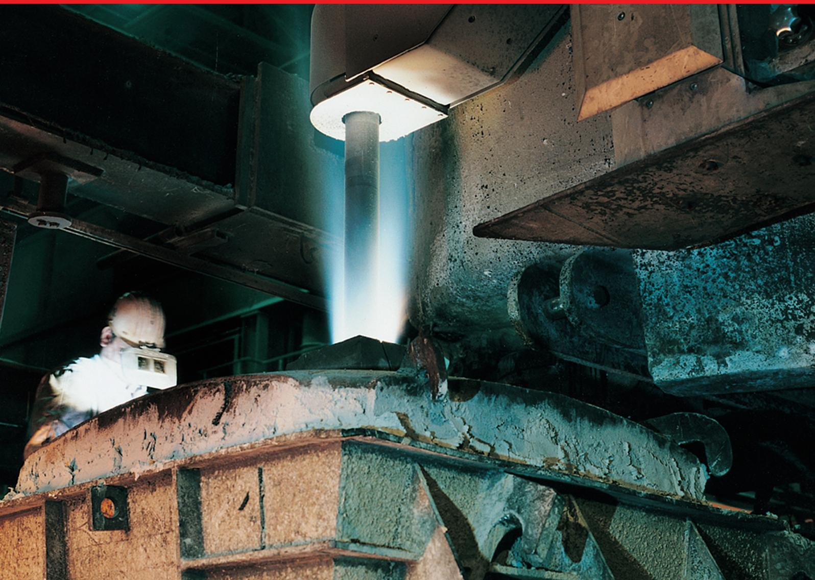
For the heating of liquid steel during continuous casting, INDUGA offers systems which heat the melt using electric plasma arcs. Depending on the application, the system can be operated with AC or DC power and special graphite electrodes. Excellent temperature control and a clean, carburisation-free heating are assured in all cases.
