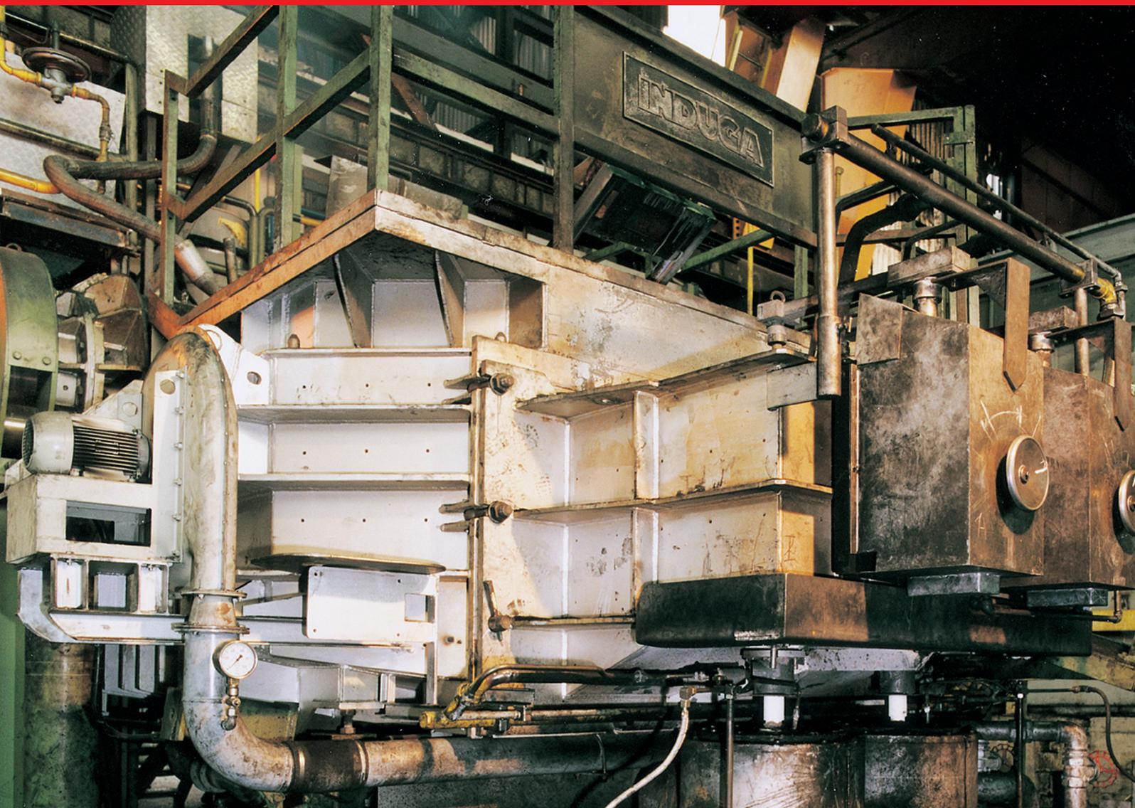
The demands made on the quality of the melt for the production of continuous cast semi-finished products are rising continuously. In order to guarantee the maximum utilisation of the casting lines, an adequate volume of liquid metal ready for casting with a constant temperature has to be supplied. To meet these demands, INDUGA has continuously optimised the induction heated holding furnace with receiver.
